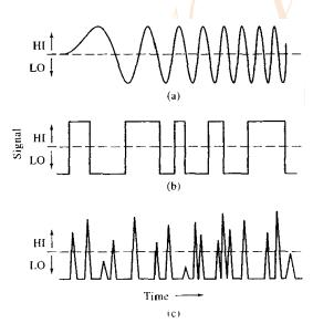
Information is stored in the time domain as the time relationship of signal fluctuations, rather than in the amplitudes of the signals. The time relationships between transitions of the signal from HI to LO or from LO to HI contain the information. The time between successive LO to HI transitions is called the **period** and the time
